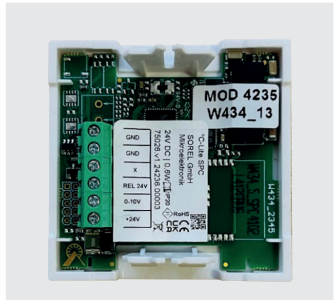
Figure 2. Underside of controller showing terminal blocks
